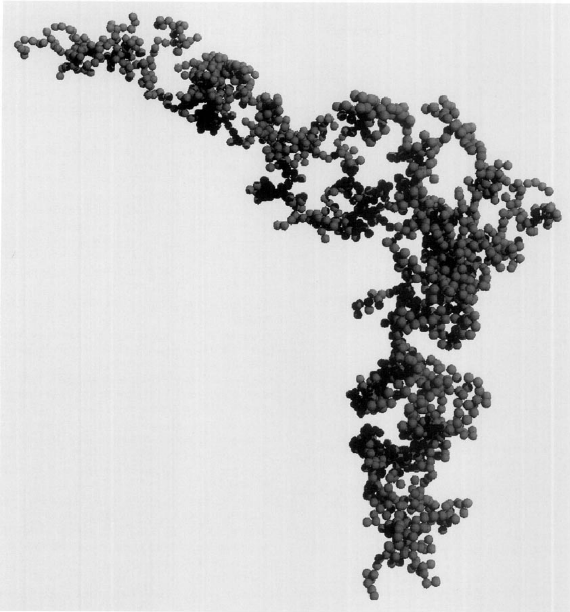
FIG. 12. Ray-traced diagram showing the configuration of the largest aggregate at the end of the model (v) run. The aggregate contains 1811 particles and has a fractal dimension nearly equal to 2. Note that apparent size differences between spheres in this diagram are simply a consequence of the 3D viewing geometry.
