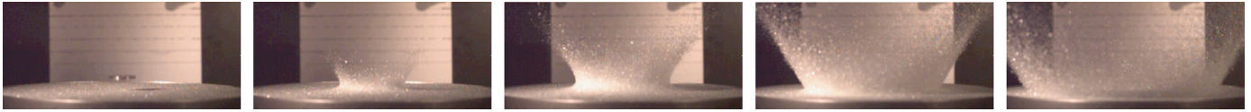
Fig. 2. Successive frames showing an experiment that uses a flat projectile impacting into a target comprising 0.5 mm glass beads, producing a symmetrical ejecta plume.
