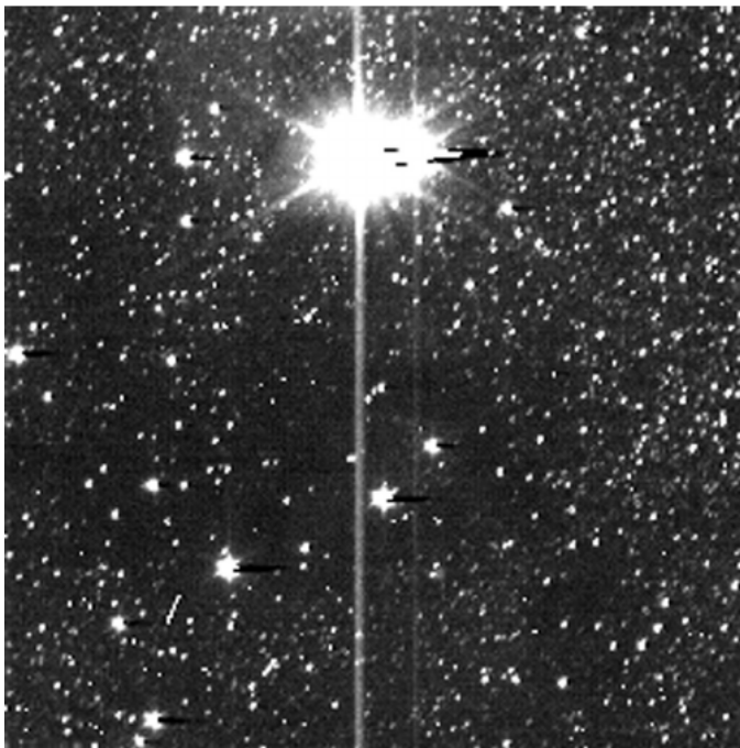
Fig. 6. The first 4 \times 4 LORRI image, lor_0296651467, in the P-29 hazard-search sequence is shown to exhibit the typical features present in the search imagery. The exposure is 10 s. Note the heavily crowded background from the Milky Way bulge. Hot pixels and cosmic-ray events are also evident. Pluto and Charon are both heavily overexposed. The vertical streaks spanning the full frame are charge left over from an incomplete frame-transfer correction due to the saturated centers of Pluto and Charon. Both objects, as well as the brightest stars, also exhibit “amplifier undershoot” tails to the right of the core of the images, which pull the local signal below the sky level.
