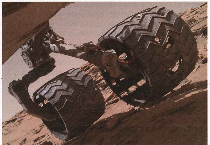
▲ HOLEY ROLLER Despite their careful design, Curiosity's wheels became increasingly punctured by pointy, immobile rocks the rover drove over. (The regular-shaped rectangular holes, on the other hand, are intentional: Scientists use the marks they leave in the rover's tracks to verify the distance the rover has traveled.)
