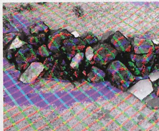
▲ NAVIGATING OBSTACLES These images provide an example of what the navigation camera aboard NASA's 2020 rover sees. On the left is a pile of rocks as seen by the rover, from 15 meters (roughly 50 feet) away. The right-hand picture shows how camera data reveal the pile's 3D contours. Using the 3D information, the rover team can plan precise travel and arm movements.
