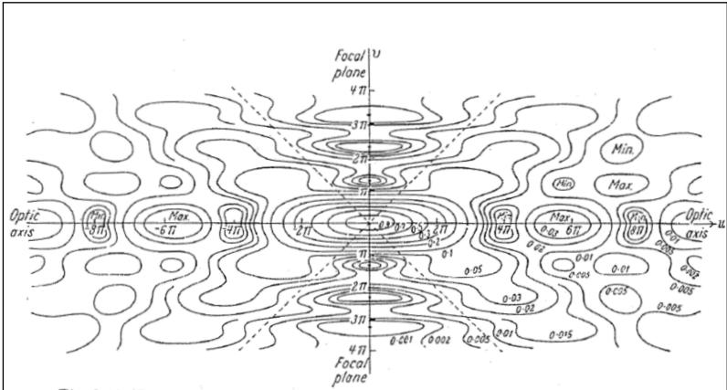
Fig. 8.41. Isophotes [contour lines of the intensity I(u, v)] in a meridional plane near focus of a converging spherical wave diffracted at a circular aperture. The intensity is normalized to unity at focus. The dotted lines represent the boundary of the geometrical shadow. When the figure is rotated about the u-axis, the minima on the v-axis generate the AIRY dark rings.
