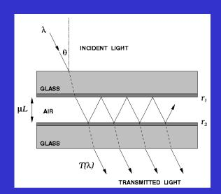
Etalon: two parallel flat semitransparent mirrors separated by a fixed distance L
