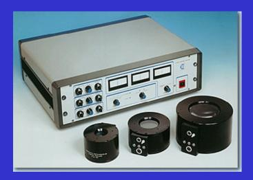
This system acts as a narrowband filter, producing concentric rings at each wavelength
