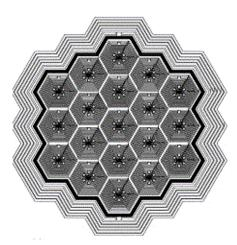
Fig. 4. SDD array made of 19 hexagon cells of 5 mm<sup>2</sup> (Lechner et al. 2001). The overall size of the detector is just about  $1 \text{ cm}^2$ .
