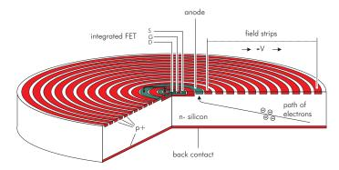
**Fig. 2.** Schematic cross section of a cylindrical Silicon Drift Detector (SDD). Electrons are guided by an electric field towards the small collecting anode located at the center of the device. The first transistor of the amplifying electronics is integrated on the detector ship (drawing kindly provided by P. Lechner).
