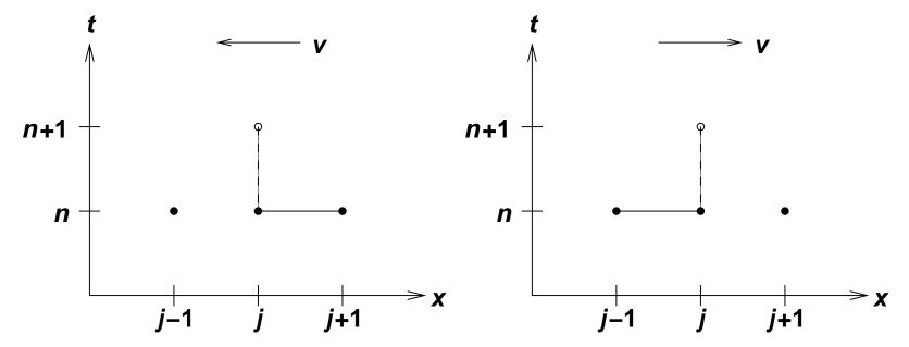
Upwind difference is only first order in space. Still, it has lower transport error than second-order centered difference. Better? Can construct higher-order upwind difference schemes...
