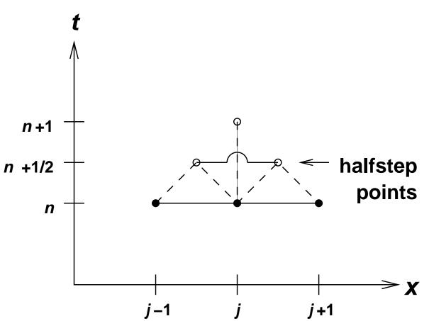
Fixes dissipation and mesh drifting but introduces phase error (dispersion). Often first-order upwind scheme is as good as/better than 2<sup>nd</sup>-order L-W.
