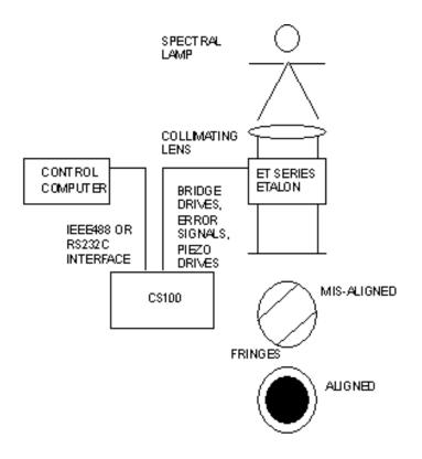
Figure 4.1Aligning the Etalon
