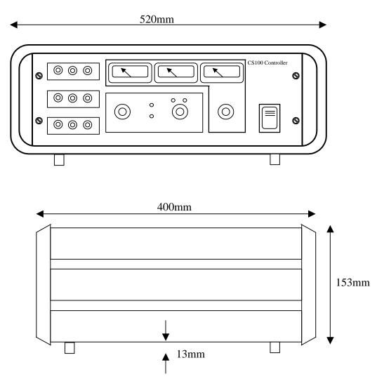
A schematic diagram of the CS100 is shown in Figure 2.3.
