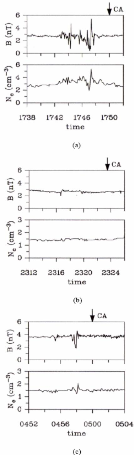
**Figure 2** Magnetic field amplitudes and electron densities of the "Phobos events" as measured by Phobos-2 during its (a) first, (b) second, (c) and third elliptical orbits. The arrows marked by CA indicate the time of closet approach to Phobos' orbital path. From [7].
