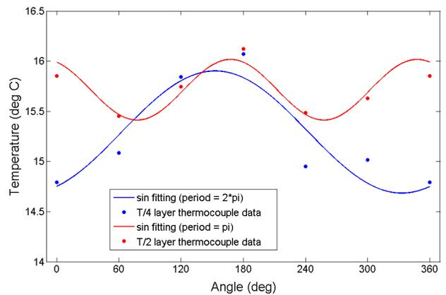
Figure 12: (above) An example of flow pattern in all the three planes at an arbitrary time during steady flow (460<sup>th</sup> minute for experiment (iii)) (below) Sinusoidal curve fitting at the same time for the bottom layer and middle layer
