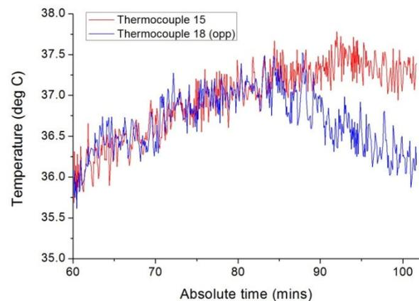
Figure 7: Readings of oppositely placed thermocouples in the middle layer showing flow separation into cold and hot plumes
