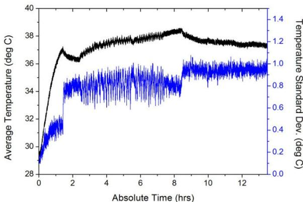
**Figure 9: Plot of mean temperature (black) and temperature variation (blue) with time**
