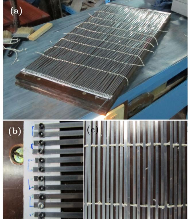
**Figure 2: Heating assembly - (a) The series of nichrome strips on the Bakelite base (b) The fixing and contacts at the strip ends (c) Alternate looping of the asbestos thread around the strips**
