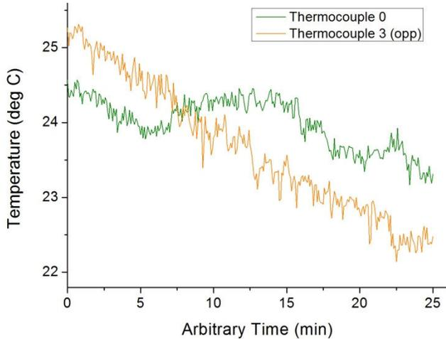
**Figure 8: Readings of oppositely placed thermocouples in the upper layer showing switching of plume position (cessation type pseudo-reversal)**
