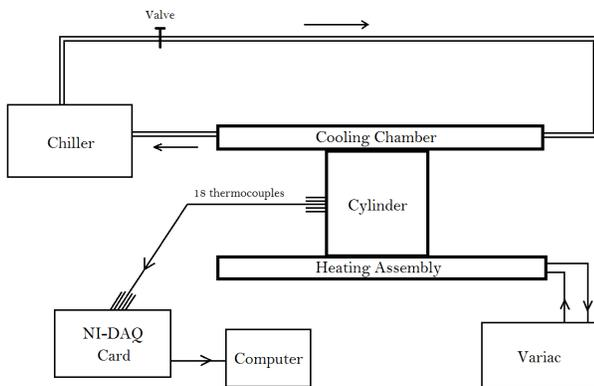
Figure 6: (above) Apparatus in running state
