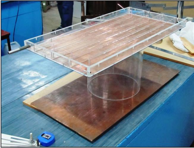
Figure 3: Top chamber assembly
