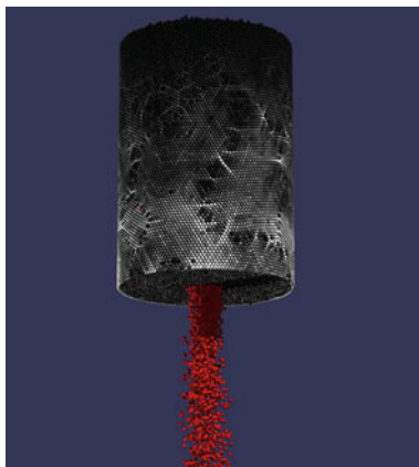
Fig. 4 Snapshot of Sim. 24 (see Table 1 for simulation parameters) showing the network of normal force distribution on particles at the hopper wall after 12.2 s of discharge. Particles under maximum stress are shown in white; darker particles feel less stress; red particles (mostly flowing out the bottom) feel no stress. See Online Resource 2 for an animation of the discharge of Sim. 24 (the duration of the animation reflects the simulated duration of the discharge). (Color figure online)
