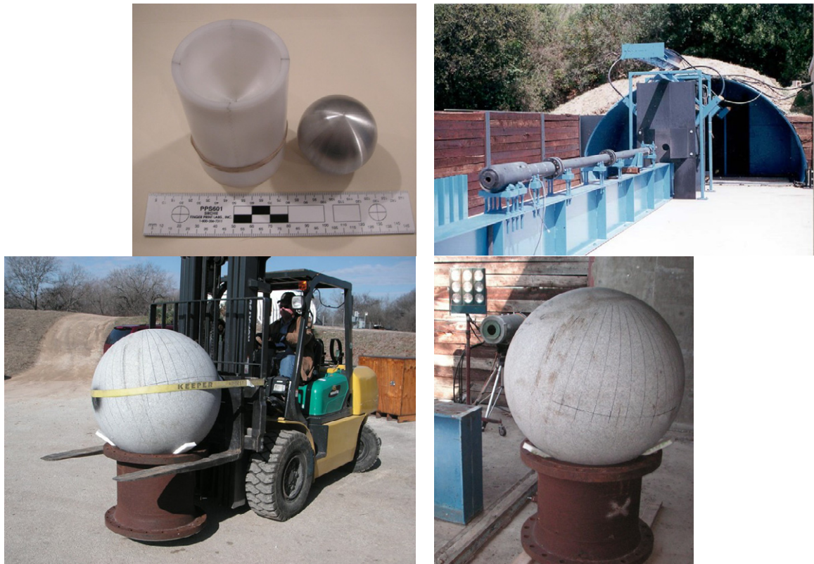
Fig. 1. Images from the experimental set-up: upper left shows the 4.45-cm diameter aluminum sphere with Lexan sabot; upper right shows SwRI's 50-mm powder gun mounted on a rail with x-ray systems (not utilized in these experiments); lower left shows fork lift moving the first test granite sphere; lower right shows the granite sphere on stand on top of wooden 2×4s.
