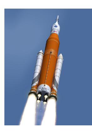
upper stage. The next planned evolution of the SLS, Block 1B, will use a new, more powerful Exploration Upper Stage (EUS) to enable more ambitious missions and deliver a 105-metric-ton (115-ton) lift capacity. A later evolution, Block 2, would replace the current five-segment boosters with a pair of advanced solid or liquid propellant boosters to provide a 130-metricton (143-ton) lift capacity. In each configuration, SLS
