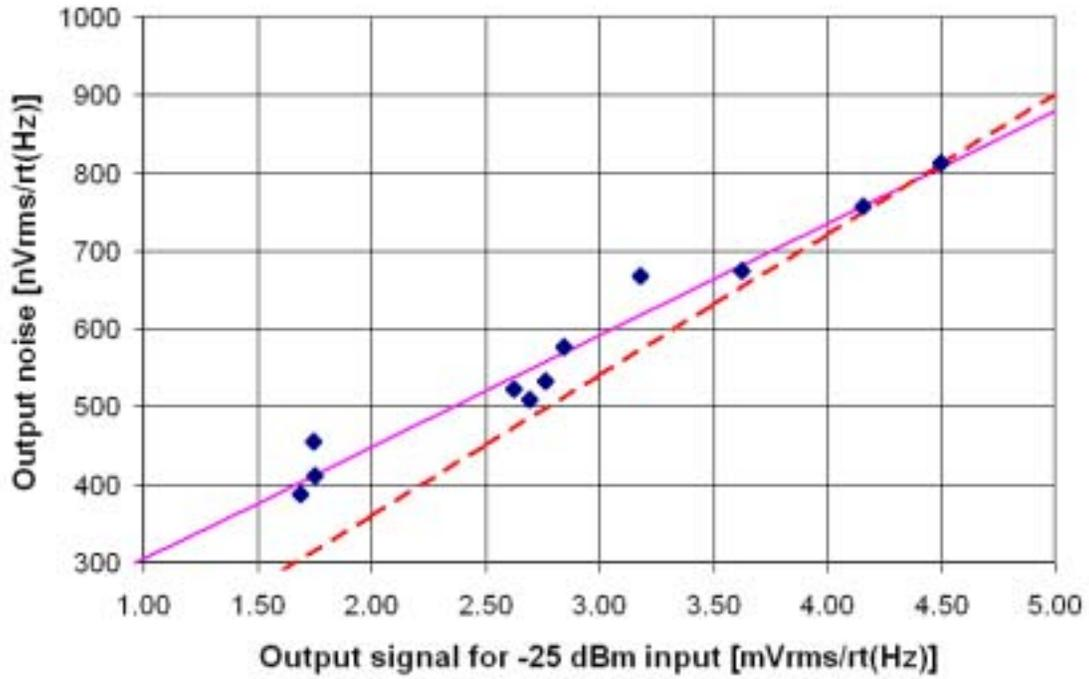
Figure 3: Output noise vs. output signal, or responsivity, (points) for -25 dBm input power level. The solid line is a linear fit to the data and the dashed line would be perfect scaling of noise with response, normalized to the highest point. The noise decreases somewhat more slowly than the responsivity.
