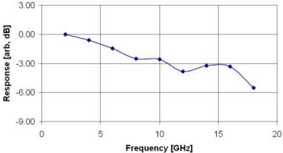
Figure 2: Representative multiplier response vs. frequency.
