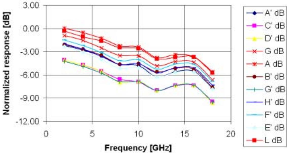
Figure 1: Response vs. frequency for a sample of 11 multipliers. Multipliers without primes are from the prototype run; those with primes are two samples each from each wafer in the June 2003 run. The response of the three multipliers from the prototype run is above the response of the eight from the June fabrication.
