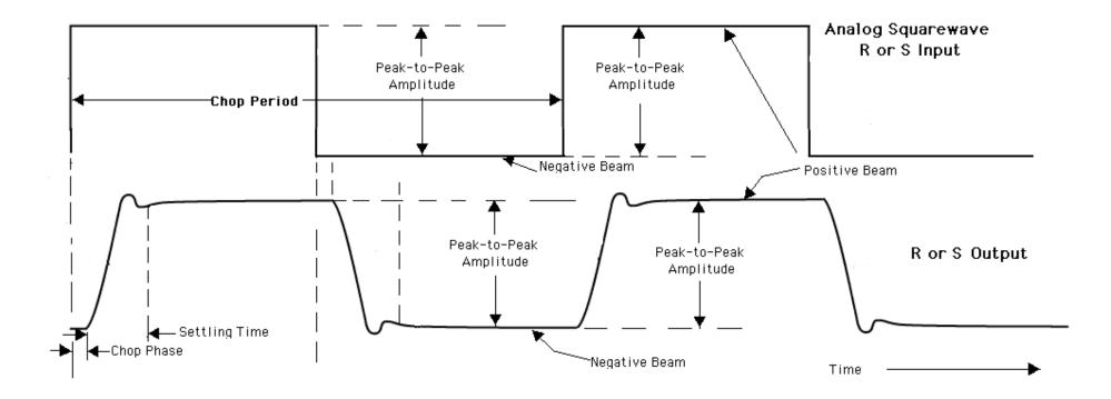
Actual 3.5 Hz external analog chop waveform with Amplitude = 9.7 arcmin at Chop Angle= 45 deg
