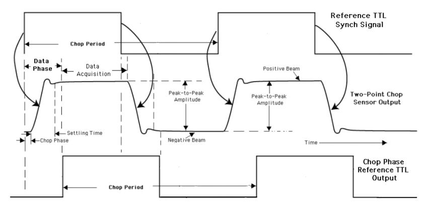
Chop Phase Ref TTL Output corresponds to Ref TTL Output but with a phase lag equal to the "Data Phase" as determined by the PI and entered using the MCS command TCM\_DES\_PHASE.
