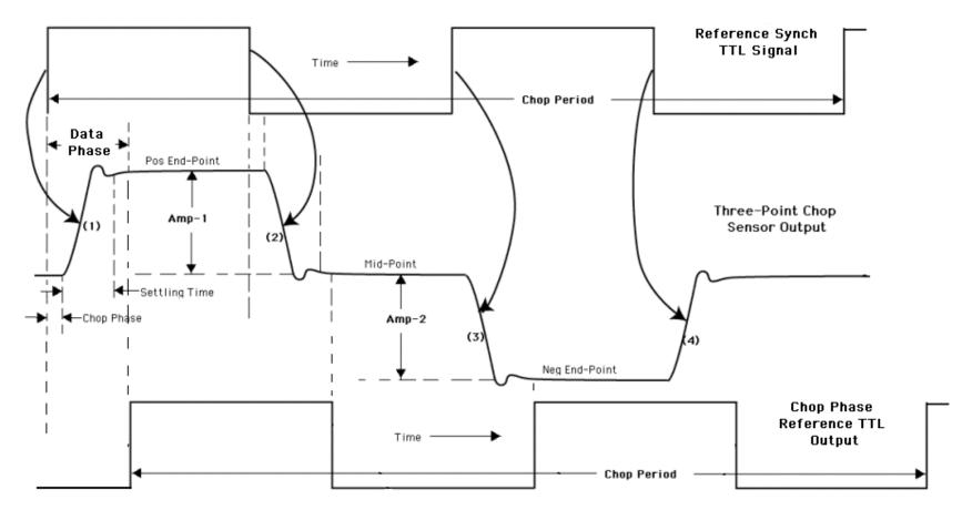
Chop Phase Ref TTL Output corresponds to Ref TTL Output but with a phase lag equal to the "Data Phase" as determined by the PI and entered using the MCS command TCM\_DES\_PHASE.
