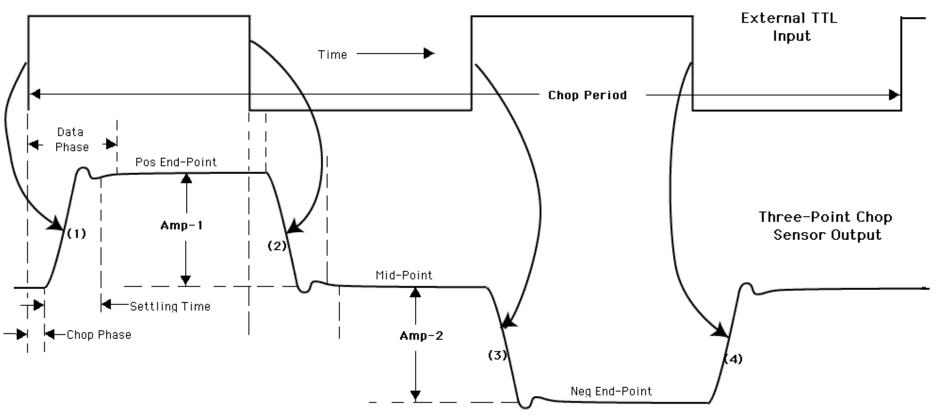
DCR-0106.R1: Polarity phasing between the sync-in TTL signal and the chop directions shall be provided. CSEM states: chopper always starts (or re-starts) with TTL= 1 triggering a positive end-point. After a start, then TTL=0 always corresponds to a mid-point, and TTL=1 either a positive or negative end-point, depending on the place in the sequence. If chopper/synchronization stops for some reason, a "re-start" will automatically force a TTL=1 triggering a positive end-point. 8
