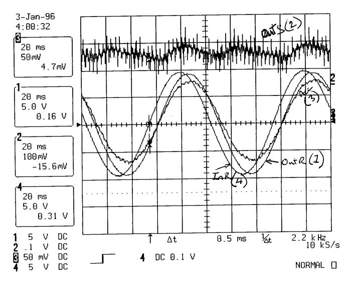
Note: Curve 3 is the output of an accelerometer on the dummy mirror. This is almost in phase with the R analog output, implying little time lag between mirror motion and the analog output signals
