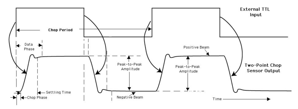
DCR-0106.R1: Polarity phasing between the sync-in TTL signal and the chop directions shall be provided. CSEM states: chopper always starts (or re-starts) with TTL= 1 triggering a positive end-point. After a start, then TTL=0 corresponds to a negative end-point, and TTL=1 a positive end-point. If chopper/synchronization stops for some reason, a "re-start" will automatically force a TTL=1 triggering a positive end-point. No 180 degree phase ambiguity.
