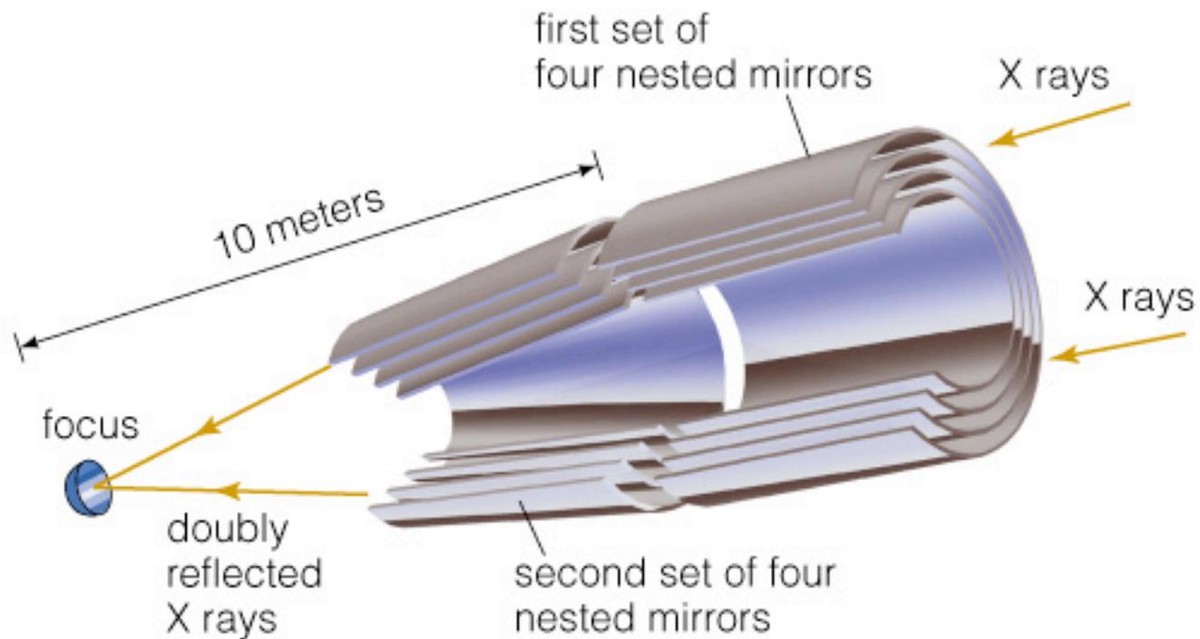
Mirror elements are 0.8 m long and from 0.6 m to 1.2 m in diameter.
