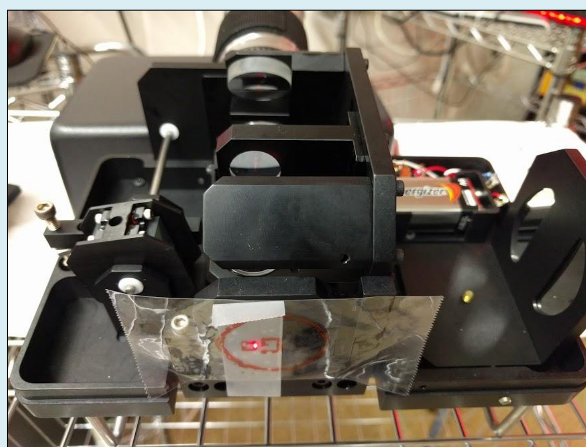
The laser shining into the spectrometer projected onto a piece of tape where the camera would be showing where the CCD chips are. Photo taken by Lucas Bloom
