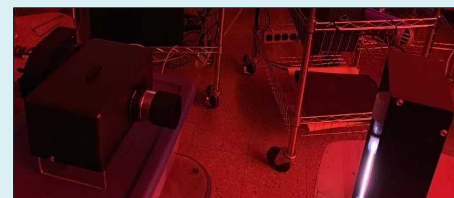
An element tube shining light into the spectrometer where it is diffracted into that element's unique spectral pattern. Photo taken by Lucas Bloom
