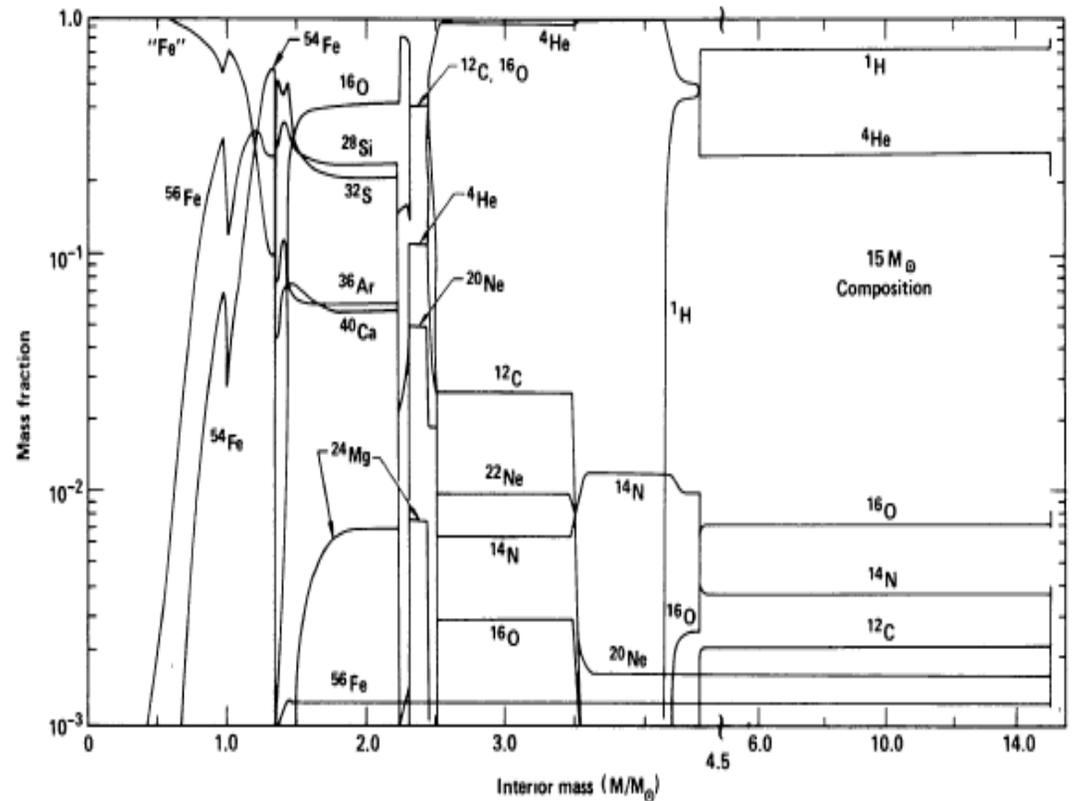
Figure 1 Structure and composition of a  $15M_{\odot}$  presupernova star at a time when the edge
