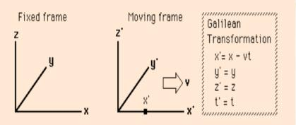
The primed frame moves with velocity v in the x direction with respect to the fixed reference frame.
