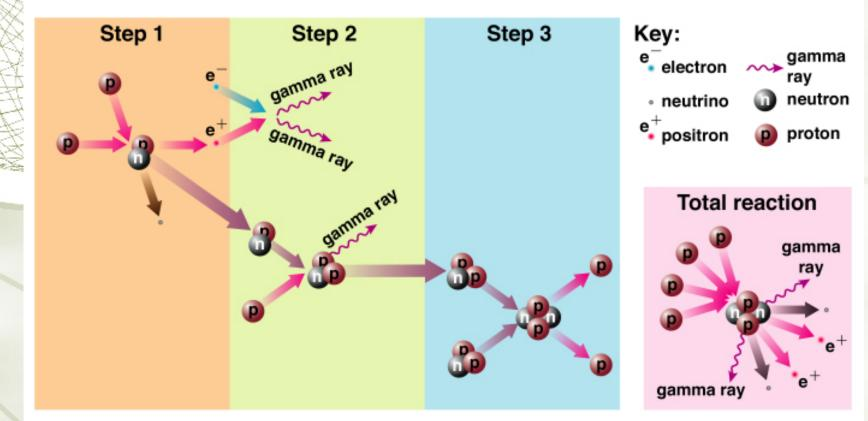
~3Mev released per He<sup>4</sup>created mass on field and 2002602AMU (1AMU=1.6603x10<sup>-27</sup>kg) Proton mass=1.00727AMU  $\Delta$ =0.00264AMU ;**0.7% efficient** E=Mc<sup>2</sup>=3.95x10<sup>-12</sup> watts; if all into energy-but some is carried away in neutrinos 25
