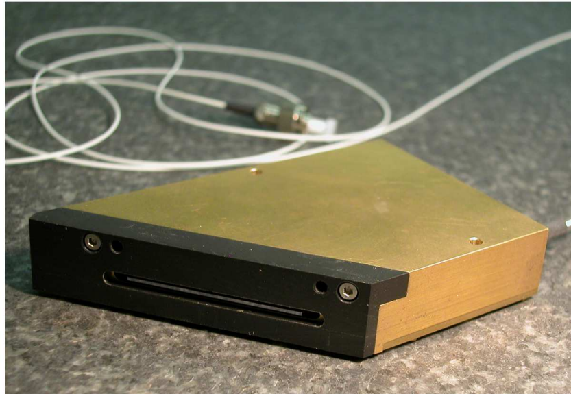
Fig. 1. Top: schematic of the AWG chip. Bottom: photograph of the IPS prototype. In this prototype device, the output array waveguides (standard in commercial devices) have been removed, the output facet has been polished back to the focal surface, and the chip packaged. The fiber input is at the rear of the image, and the polished flat output facet at the front. The open face of the chip is \sim 38\text{mm} in length. The active area is \sim 3\text{mm} across, and is situated at the centre of the polished face.
