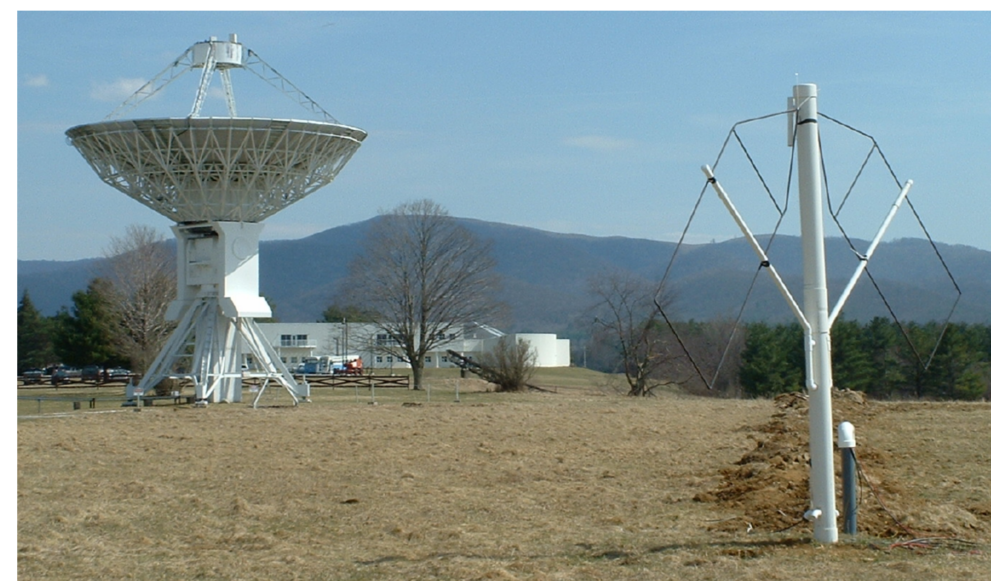
FIGURE 1: View of the Low Frequency Spectrometer (right) and the 13.7 m antenna at Green Bank, WV. Upgrades will add a 300–850 MHz feed and an 80–350 MHz log-periodic antenna on the 13.7 m antenna feeding dual polarizations to a Callisto spectrometer supplied by ETH/Zürich, and later replace the Erickson antenna with a set of four dipoles.
