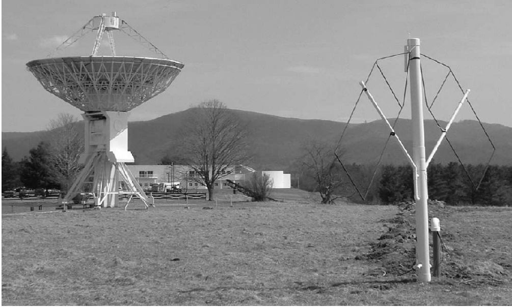
Figure 1. View of the Low Frequency Spectrometer (right) and the 13.7 m antenna at Green Bank, WV. Upgrades will add a 300–850 MHz feed and an 80–350 MHz log-periodic antenna on the 13.7 m antenna feeding dual polarizations to a Callisto spectrometer supplied by ETH/Zürich, and later replace the Erickson antenna with a set of four dipoles.
