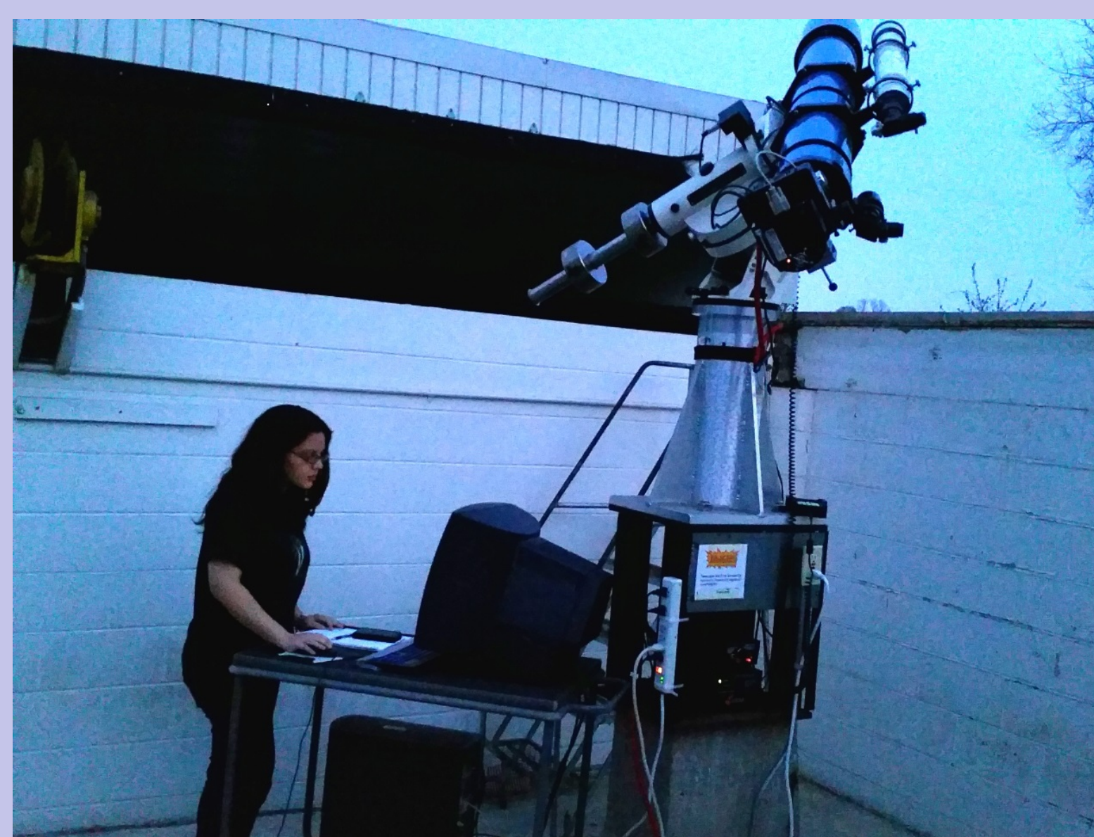
Left: Me taking flat field images with the 7-inch telescope at the UMD observatory
