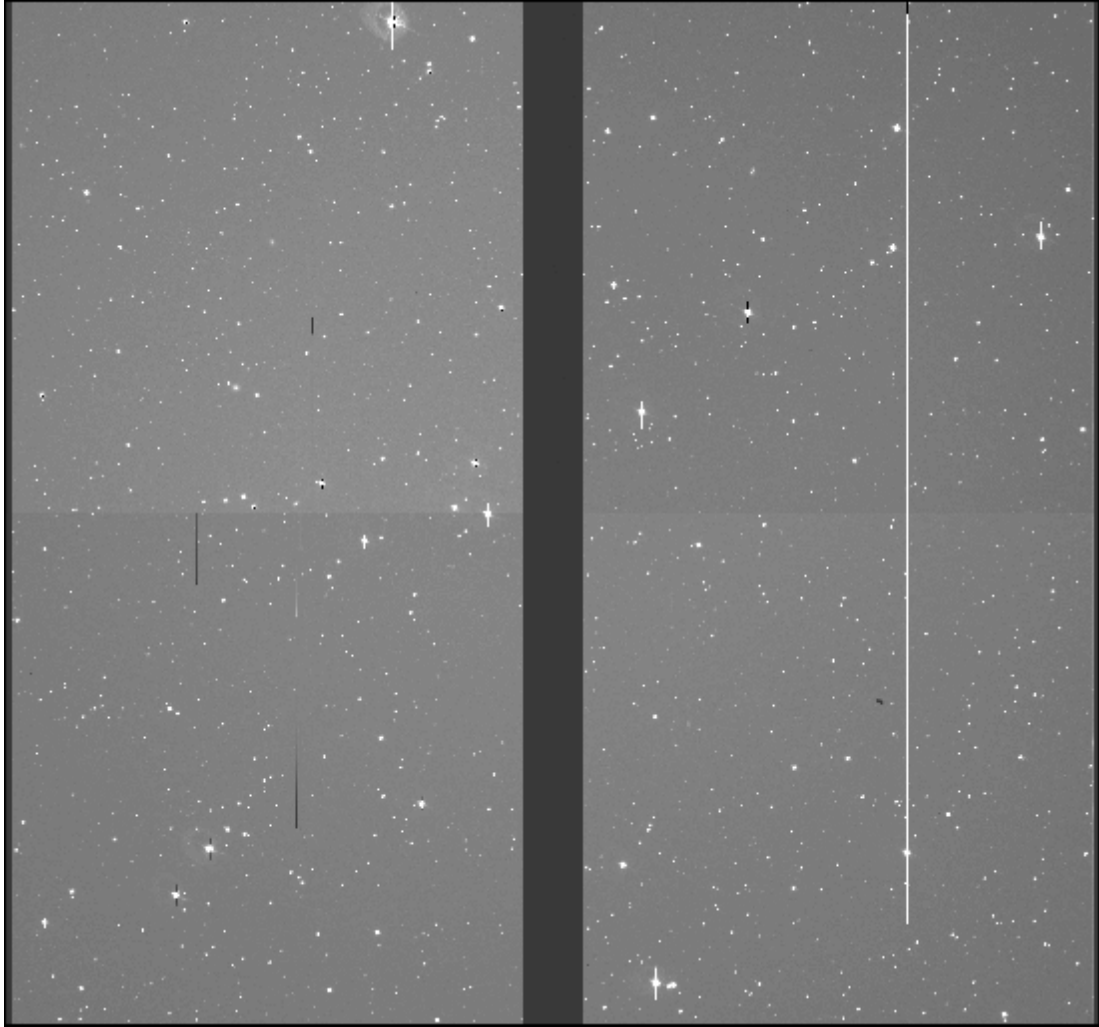
Figure 2.2: Example of the raw data. This is field F2140-45a, the first observation of the survey. Notice that the quadproc format places the overscan region in the center of the image to facilitate trimming. The few columns with no data on the left and right edges of the frame are removed in the trimming step.
