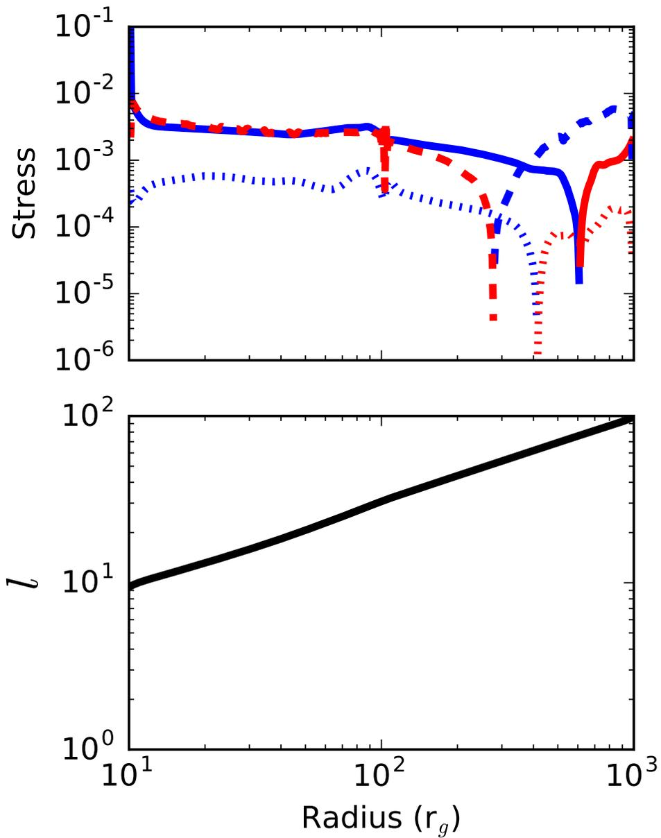
Figure 3.9: Top panel- Radial profiles of angular momentum advection (dashed line),  $r - \phi$  viscous stress term (solid line), and  $\theta - \phi$  term (dotted line) integrated through a shell at a given radius. Blue indicates a negative quantity and red indicates a positive quantity. Bottom Panel- Radial profile of time averaged specific angular momentum.
