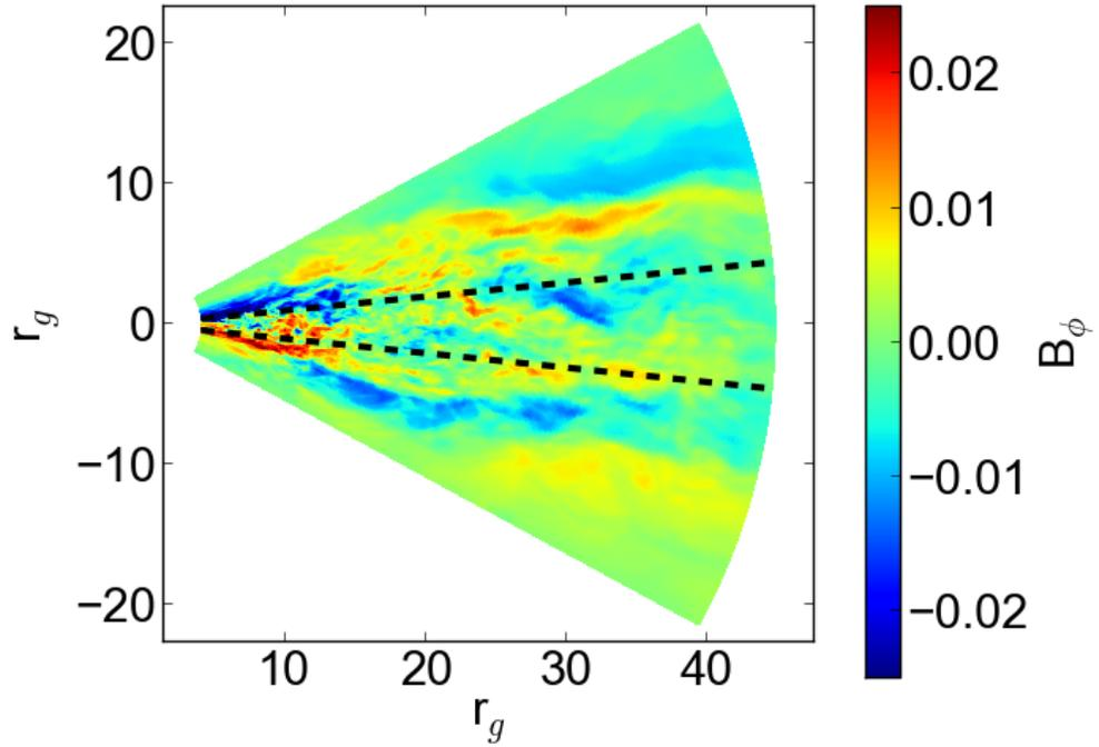
Figure 2.9: Azimuthally averaged  $B_\phi$  at  $t = 3.7 \times 10^4 GM/c^3$ . Within the disk midplane the fluctuations in  $B_\phi$  are largely random. Large, stratified regions of coherent magnetic field develop in the corona as buoyancy lifts highly magnetized gas vertically and regions of similar polarity grow through magnetic reconnection. The coronal regions are symmetric across the midplane, but have opposite polarity.
