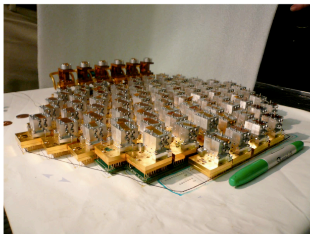
Fig. 6. (left) The QUIET W-band array, built from 91 integrated MMIC pseudocorrelation receiver modules. (right) Dual polarization module operating at 90 GHz Module operating in the 75 – 105 GHz range, with multiple drop in chips providing various functions including amplifiers (2 per channel), phase switches, hybrid junction for signal processing, and detectors for the various Stokes parameters.
