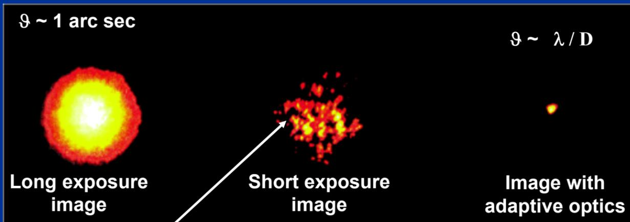
Speckles (each is at diffraction limit of telescope)
