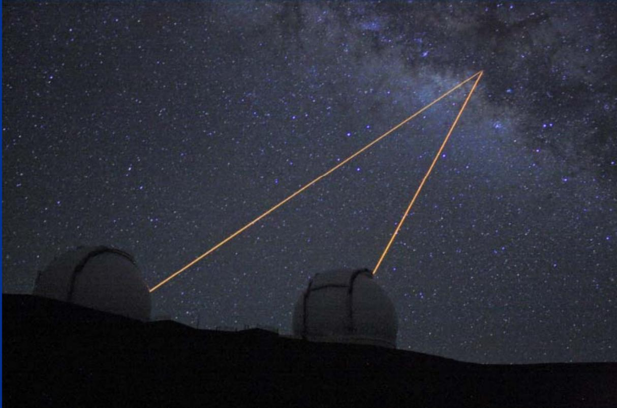
Twin beams toward the Galactic center for AO with the Keck Interferometer
