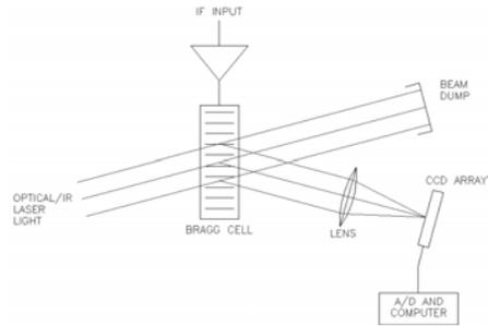
Figure 3: Schematic view of an AOS
