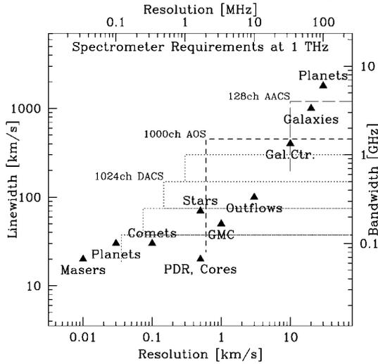
**Figure 1:** Connection between velocity and frequency scales for a set of typical sources. Frequencies scale linearly from the 1 THz (300  $\mu\text{m}$ ) example shown here.
