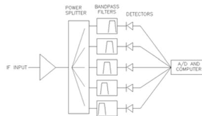
**Figure 2:** Schematic view of a filter bank spectrometer
