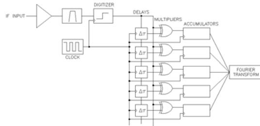
**Figure 6:** Schematic layout of a digital autocorrelator
