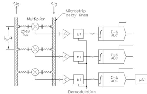
**Figure 7:** Schematic view of a WASP analog lag correlator segment.
