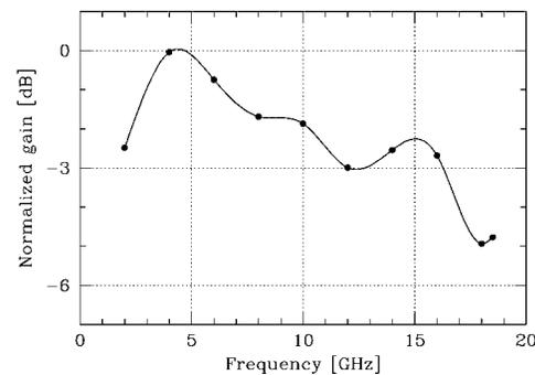
**Figure 8:** Response of a new Gilbert-cell multiplier custom MMIC for ultra-wideband analog correlators.
