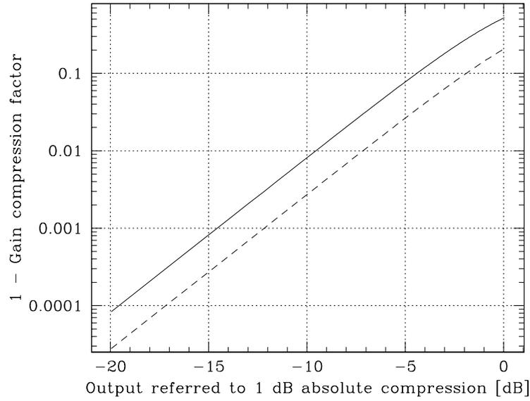
Figure 3: Gain compression factor defect limits versus output level for a device with a  $\tanh(s)$  nonlinearity. The solid curve is for small differences, the dashed curve is for large signal changes.
