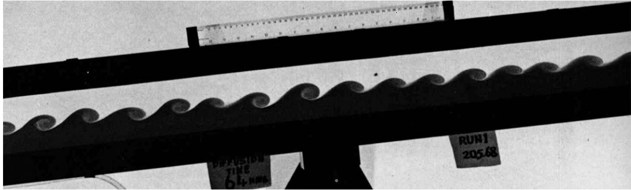
Figure 34: Experimental confirmation of the Kelvin-Helmholtz instability. In a rectangular tube, a layer of water lies on top of colored brine. The tube is suddenly tilted, setting the fluids into motion. Figure from van Dyke (1982).
