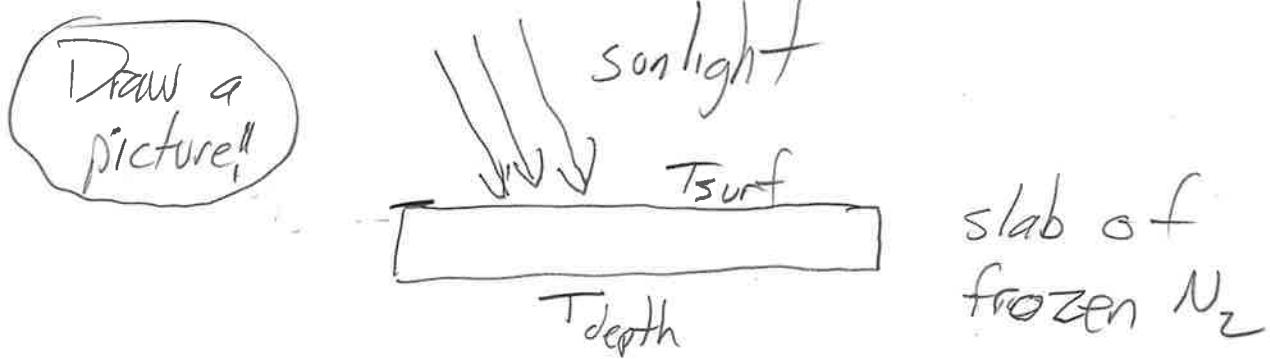
The idea is that if  $T_{\text{depth}} > T_{\text{surf}}$  the N<sub>2</sub> can vaporize at depth. The gas then rises explosively since it is less dense than its surroundings. If the pressure is large enough, liquid N<sub>2</sub> is possible too. We'll return to this possibility. But first, how can we get  $T_{\text{depth}} > T_{\text{surf}}$ ?
