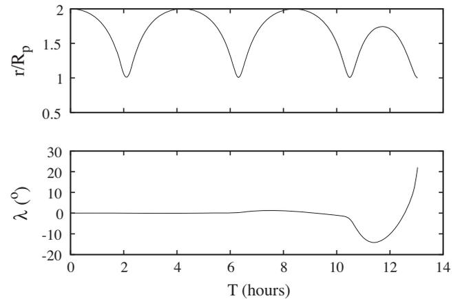
**Fig. 4.** The trajectory of a positive grain inside  $R_{syn}$  ( $r_L = 2.0R_p$ ,  $L_* = 1.908$ ,  $a_d = 0.122 \mu\text{m}$ ). Here, unlike Fig. 3, large radial motions ultimately excite vertical motions, forcing the trajectory to end with a collision at the planetary surface after just a few orbits.
