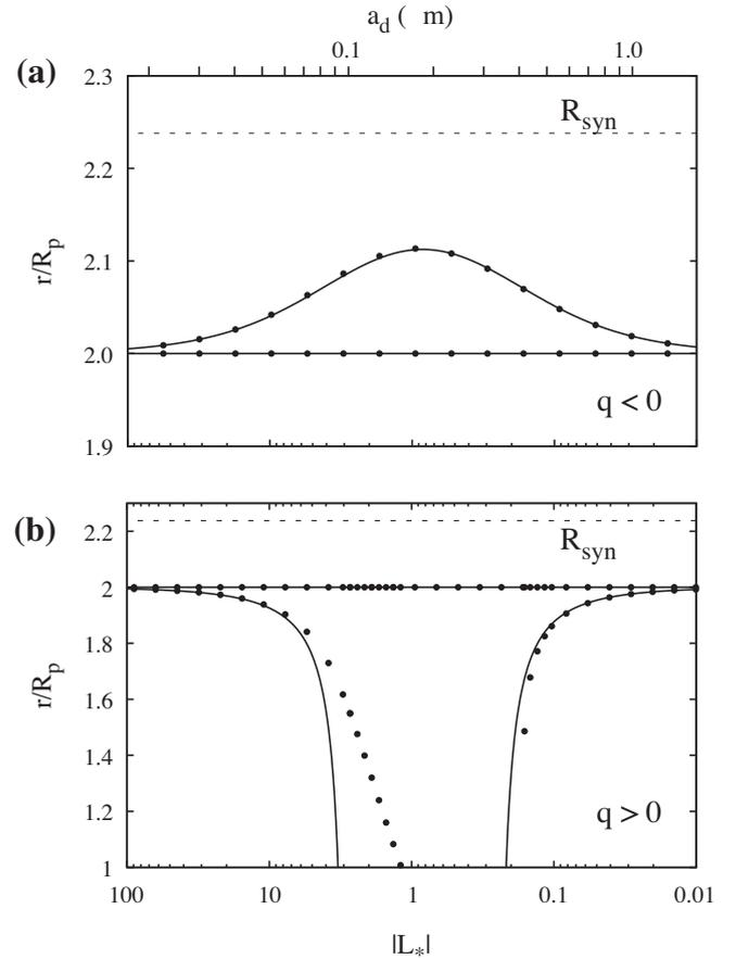
**Fig. 6.** The radial range of (a) negative and (b) positive grains launched azimuthally with the Kepler speed  $v = \sqrt{GM/r_L}$  at  $2.0R_p$ . Both numerical data (points) and the analytical results (curves from Eq. (13)) are included. The total radial excursion is twice the epicyclic radius  $r_g$ .
