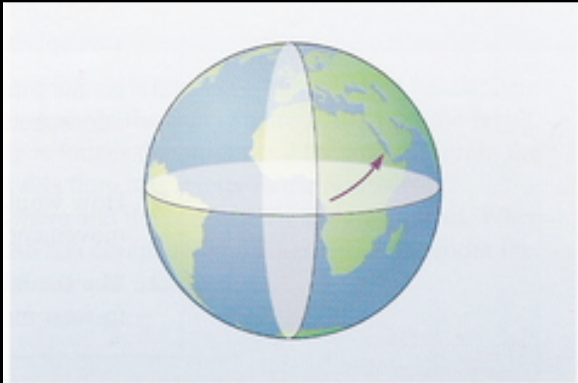
Figure 5.36 As it moves northwards, the top layer of the Hadley cell acquires an easterly motion relative to the surface of the Earth.
