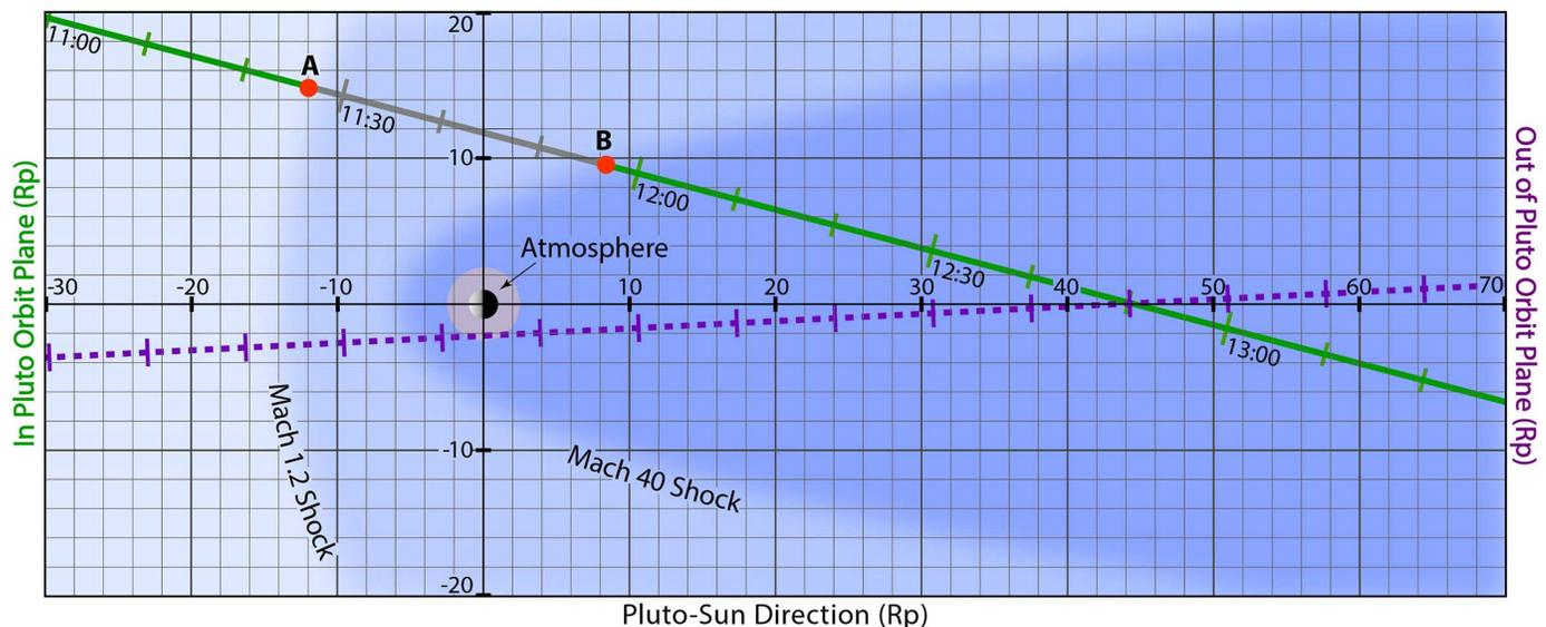
**Fig. 1. Geometry of the New Horizons trajectory through the solar wind interaction with Pluto's atmosphere on DOY 195.** Along the gray section of the trajectory between points A and B, the New Horizons spacecraft pointed the SWAP instrument's field of view away from the solar direction. The pink circle shows the extent of Pluto's atmosphere (2).
