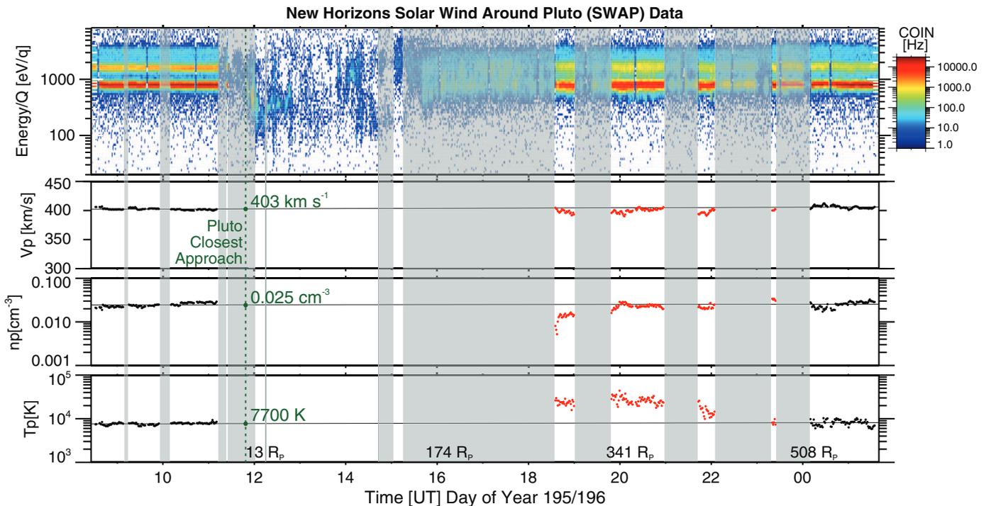
**Fig. 2. Overview of SWAP data.** Color spectrogram of coincidence count rate (COIN) as a function of  $E/q$  and derived proton flow speed, density, and temperature values for the interval surrounding the Pluto flyby. The vertical dashed green line shows the time of closest approach. Unshaded regions indicate times during which some portion of SWAP's very broad field of view was pointed within 5° of the Sun direction, and thus SWAP would be able to
