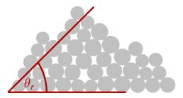
Studying these piles should give a *qualitative* view of the effect of particle shape and size distribution.
