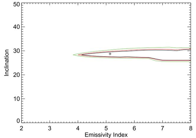
**Figure 5.** Contour plot of the emissivity index against the inclination angle, which was calculated from the REFLIONX model. The contours are plotted at 67% (black), 90% (red), and 99% (green) confidence levels. It can be seen that there is no clear degeneracy between emissivity and inclination angle.
