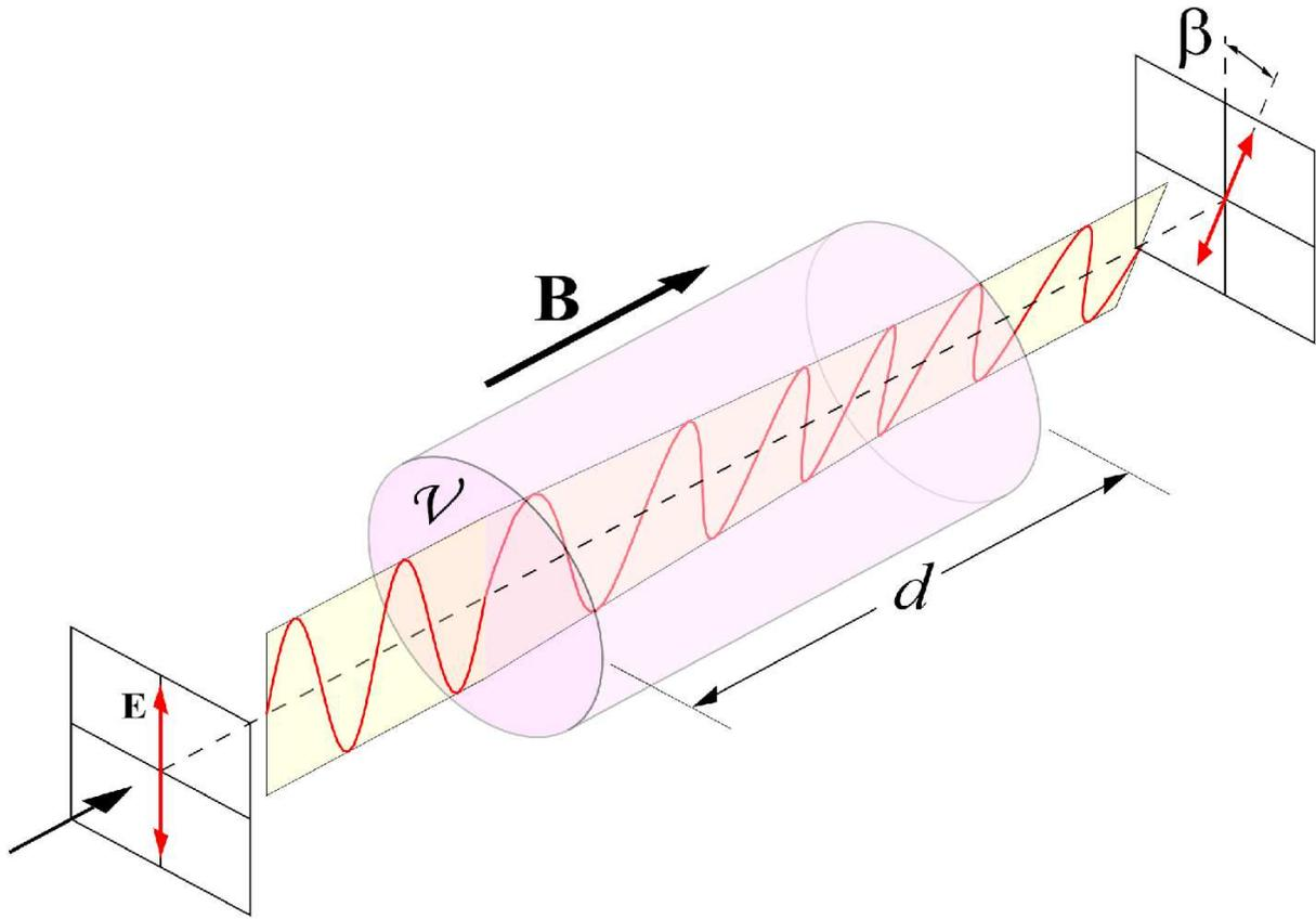
Fig. 1.— Schematic of Faraday rotation, from Wikipedia. This is for the rotation of polarization in matter, where there is a quantity  $\nu$  related to the properties of that matter. In our case, the angle  $\beta$  of rotation is proportional to the integral of the number density times the magnetic field strength along the propagation direction over the extent of the region.
