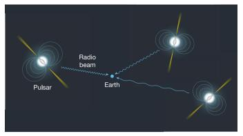
**Fig. 5** | **Operation of a pulsar timing array for the detection of low-frequency gravitational waves.** The signals from the pulsars travel through spacetime that is dynamically warped by gravitational waves, which changes the timing of the pulsars in a correlated way. Figure adapted from ref. <sup>93</sup> (Springer Nature).
