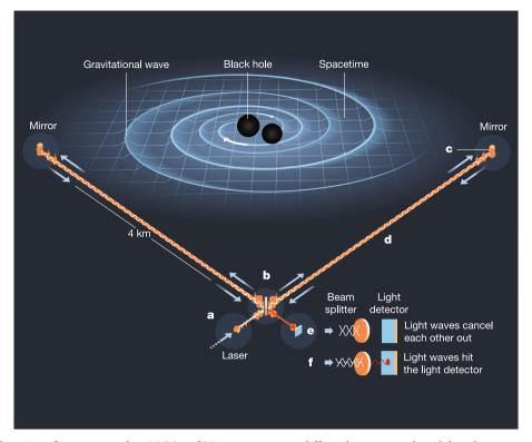
**Fig. 1** | **Operation of a laser interferometer, such as LIGO and Virgo. a**, Laser light is sent into the instrument to measure changes in the length of the two arms. **b**, A 'beam splitter' splits the light and sends out two identical beams along the arms. **c**, The light waves bounce off the mirror and return. **d**, A gravitational wave affects the interferometer's
