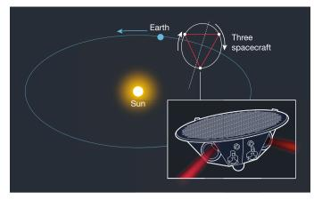
**Fig. 6** | **Representation of the upcoming space-based LISA gravitational-wave detector.** Unlike ground-based detectors, such as LIGO and Virgo, in LISA the stations are free-floating test masses in orbit around the Sun. Figure adapted from ref. <sup>93</sup> (Springer Nature).
