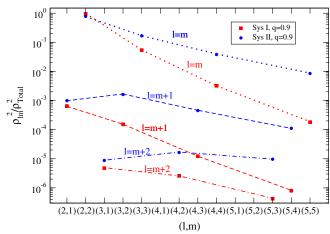
FIG. 7 (color online). Relative fraction between the squared of the SNR computed with only the  $(\ell, m)$  mode and that computed with all  $(\ell, m)$  modes. The lines connecting points are only meant to group points with  $\ell = m$  (dotted line),  $\ell = m + 1$  (dashed line), and  $\ell = m + 2$  (dot-dashed line).
