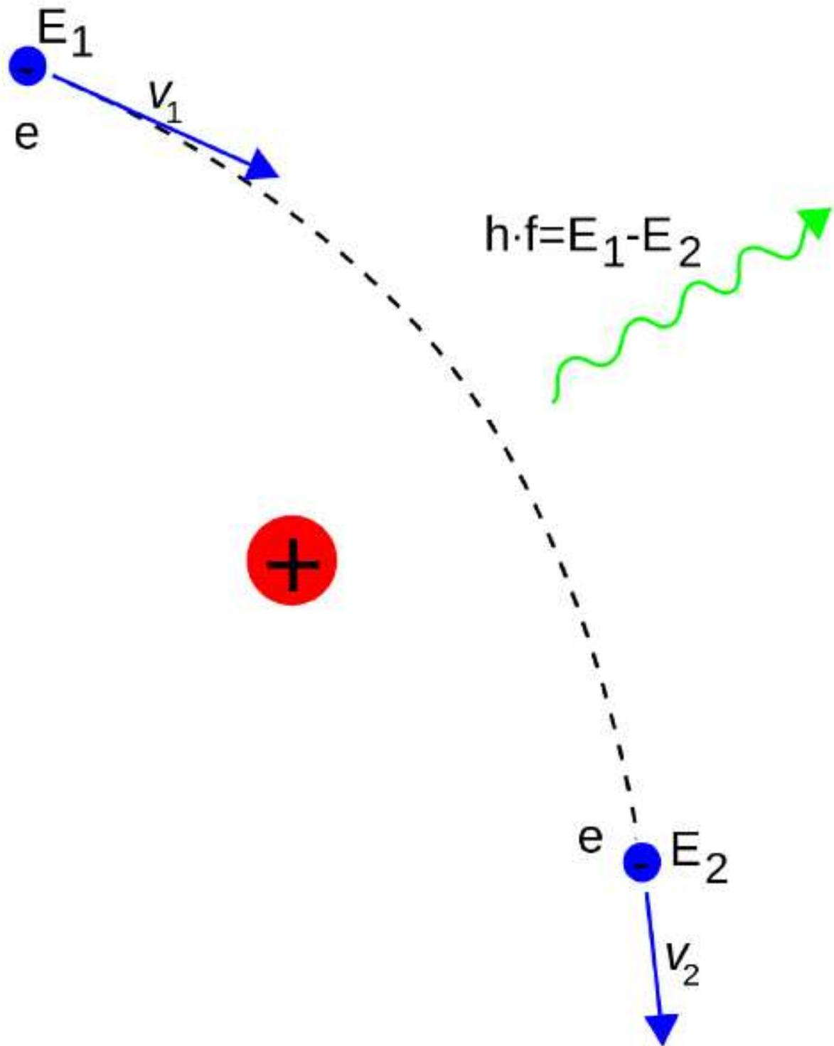
Fig. 1.— Geometry of bremsstrahlung, from Wikipedia. An electron of initial energy  $E_1$  and speed  $v_1$  as seen in the reference frame of the positive ion is deflected by the ion, radiates a photon, and ends up with energy  $E_2 < E_1$  and speed  $v_2 < v_1$  as seen in the original frame. The inverse process, in which an electron absorbs a photon as it goes by an ion, is free-free absorption.
