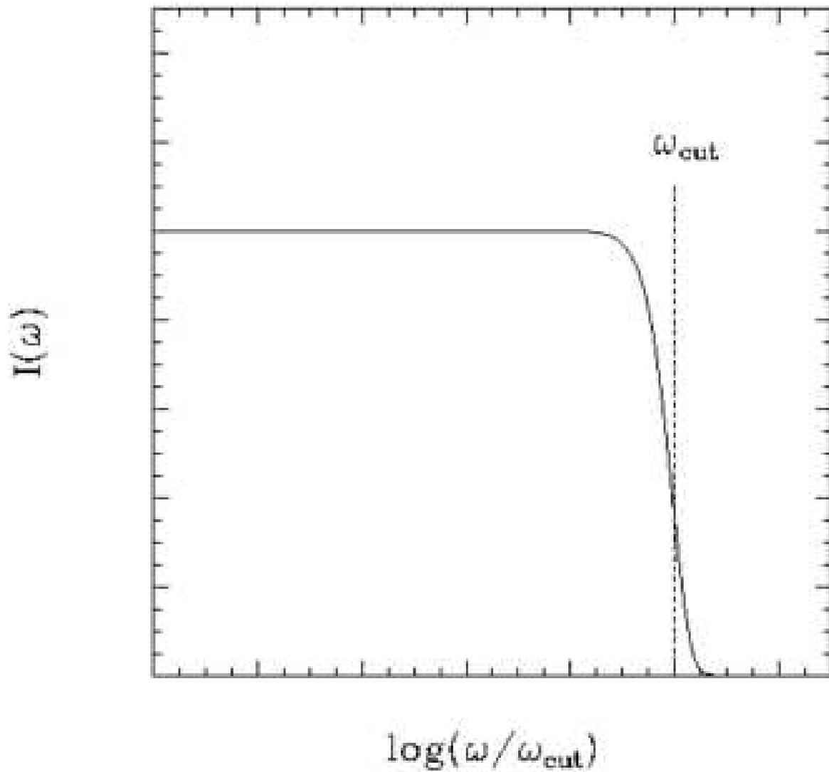
Fig. 2.— Representation of the spectrum of bremsstrahlung, from <http://www.astro.utu.fi/~cflynn/astroII/brems.gif>. The energy per volume per time per frequency is nearly constant until  $h\nu \gtrsim kT$ , after which it rolls over exponentially.
