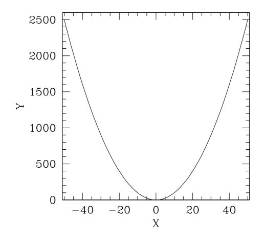
Fig. 3.— A plot of  $y = x^2$  from x = -50 to x = +50. Although the correlation is obvious, the Pearson's correlation coefficient is zero, because it measures only linear correlations.
