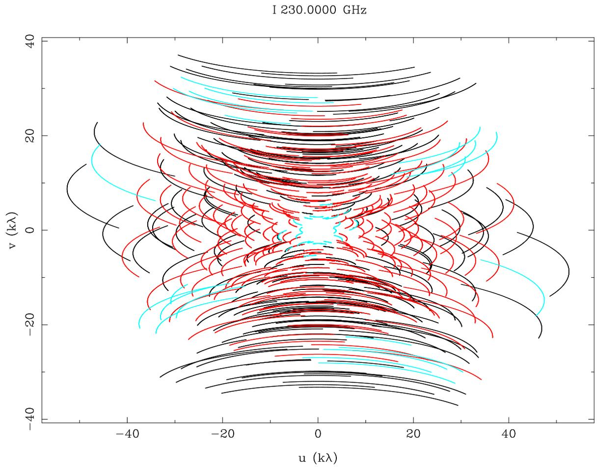
Fig. 2.—  $uv$  coverage obtained with a 23-antenna array at declination -15 degrees. The 15-antenna CARMA E configuration is shown in red. The 8-antenna SZA is in blue, and cross correlations between the two subarrays are in black.
