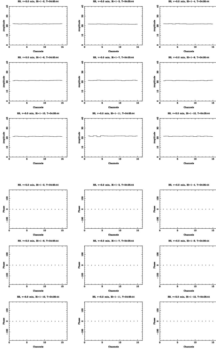
Fig. 3.— Amplitude (top) and phase (bottom) of the astronomical source (3c273) vs. channel in the 500 MHz band after noise and astronomical bandpass calibration.
