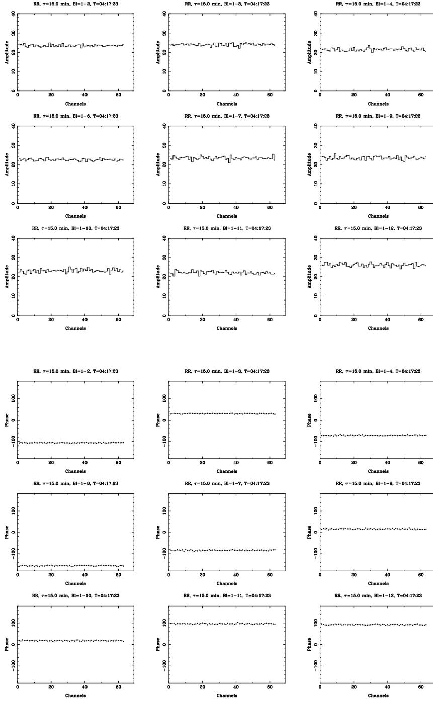
Fig. 6.— Amplitude (top) and phase (bottom) of the calibrated 31 MHz astronomical source vs. channel after another astronomical bandpass — this is done as a check to look for differences between the noise bandpass calibration technique described in Section 4.4 and a pure astronomical bandpass calibration. The flat amplitude and phase implies that there isn’t much difference between the two techniques.
