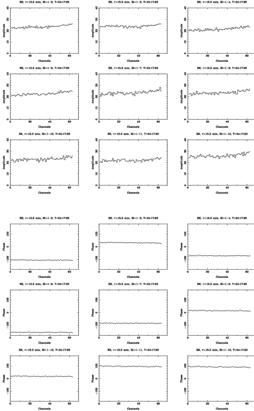
Fig. 5.— Amplitude (top) and phase (bottom) of the astronomical source (3c273) vs. channel in the 31 MHz narrowband after all bandpass calibrations have been applied. Phase offsets from zero are corrected by the gain calibration later on in the reduction process.
