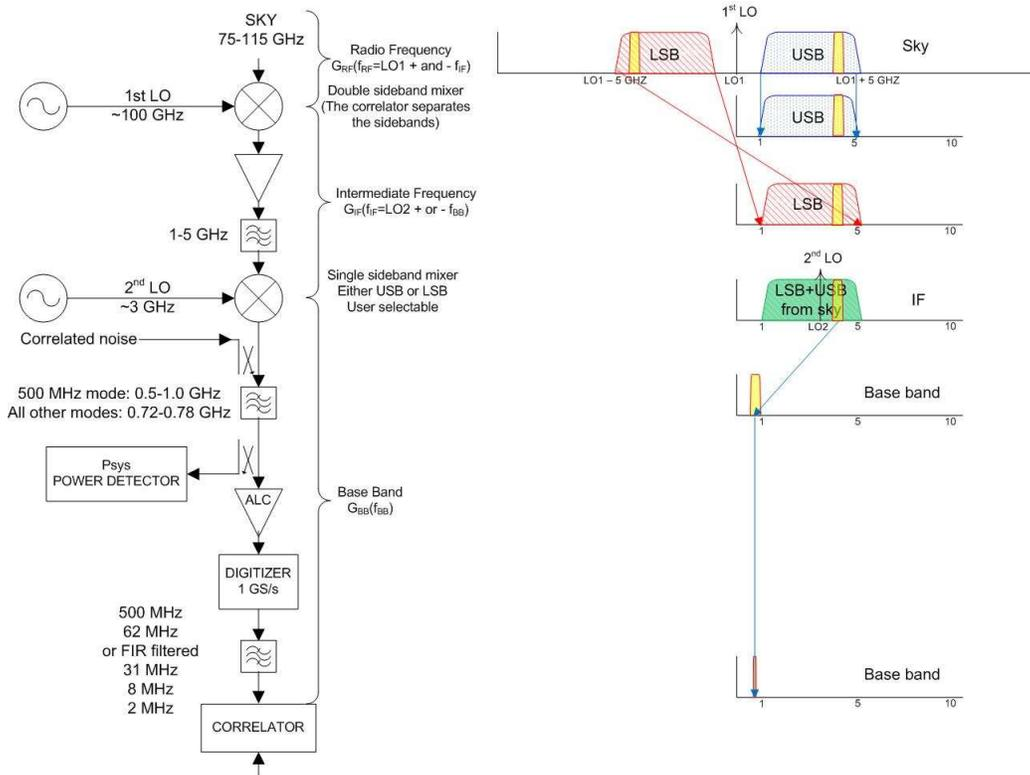
Fig. 1.— Signal path through the CARMA system.
