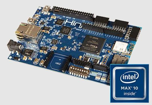
FPGAS can be thought of as generalized computer processors. They possess a vast array of logic blocks which allow for circuits to be reconfigured after production.
