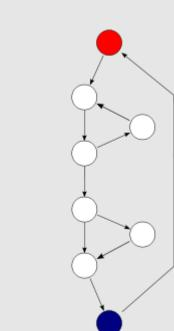
Cyclomatic Complexity Some common metrics used to judge source code are unit test coverage, line count, and comment to code ratio. A similar approach is to compute the number of independent paths through a program (cyclomatic complexity) and use this value to gauge its intricacy. The complexity of any given program can thus be measured as a
