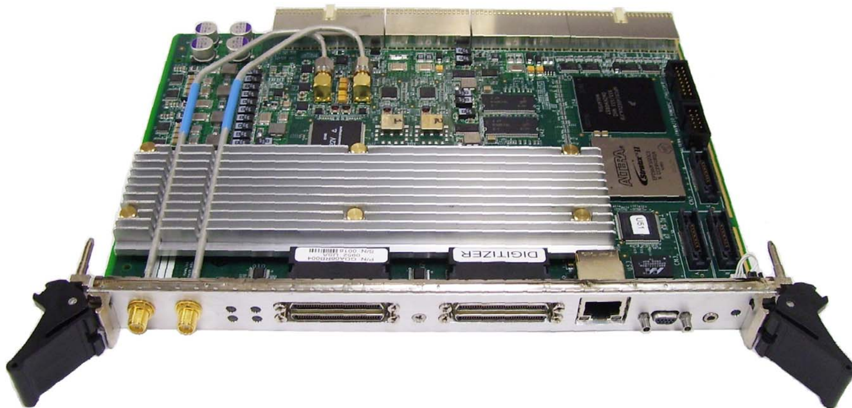
Fully assembled CARMA Digitizer Board
