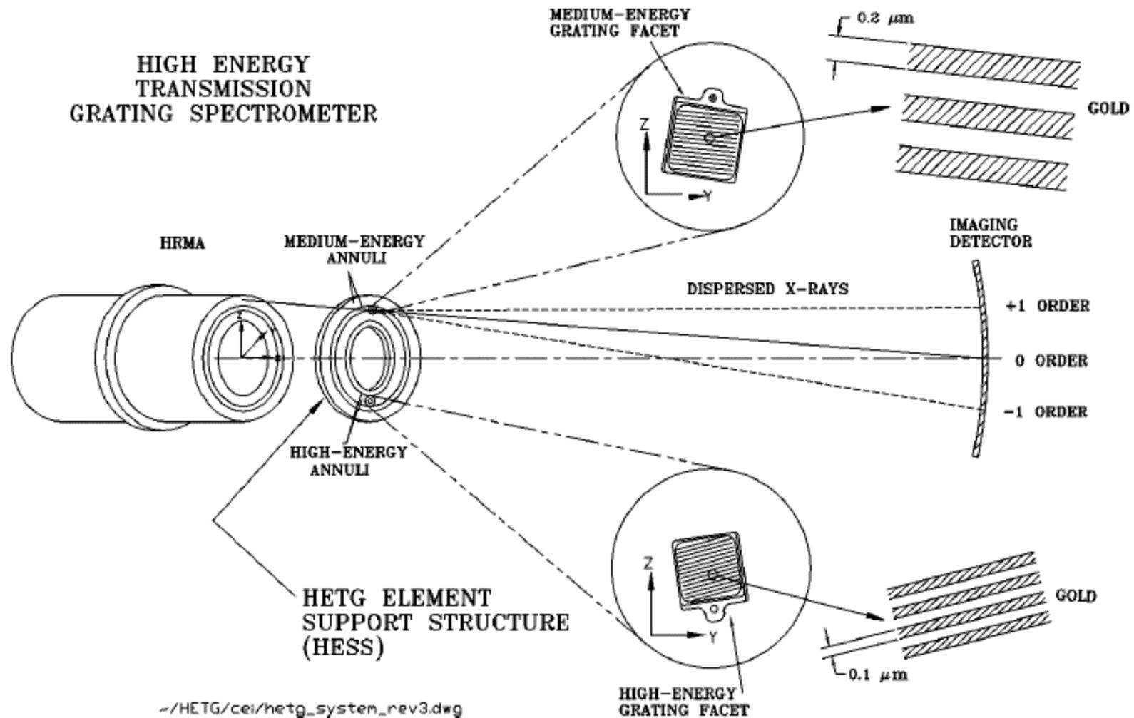
**Figure 1** Geometry of the transmission grating spectrometers on *Chandra*.
