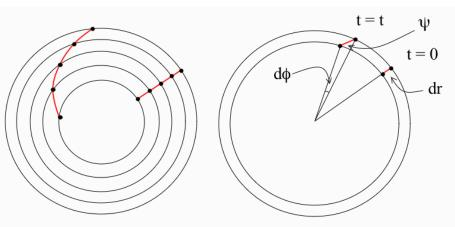
Flat rotation curve: v = const;  $\Omega = v/r$ ;  $d\Omega = v/r^2 dr$ Now,  $\phi = \Omega \times t$ , so  $d\phi = d\Omega \times t = v/r^2 dr t$ So tan  $\psi = dr / r d\phi = dr / [(v/r) dr t] = r / vt = 1/\Omega t = 1/\phi$
