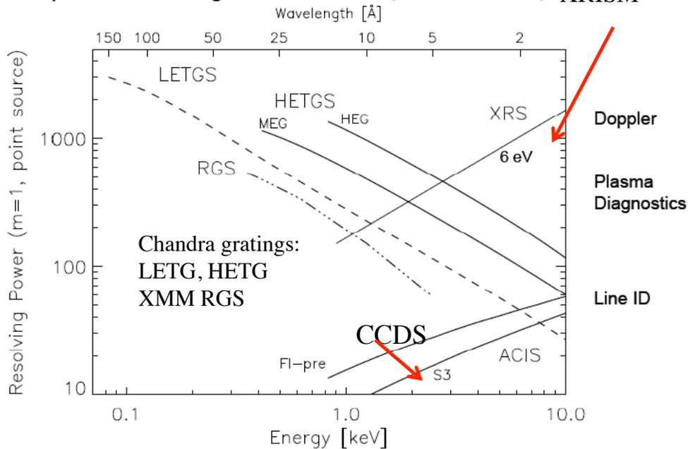
$$\text{Spectral Resolving Power} = E/\Delta E = \lambda/\Delta\lambda$$
