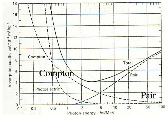
Figure 4.16. The total mass absorption coefficient for high energy photons in lead,
